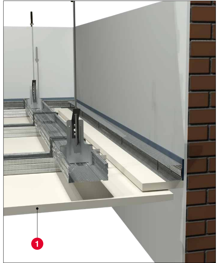
Fig. 6. Expansion joint of a suspended ceiling
