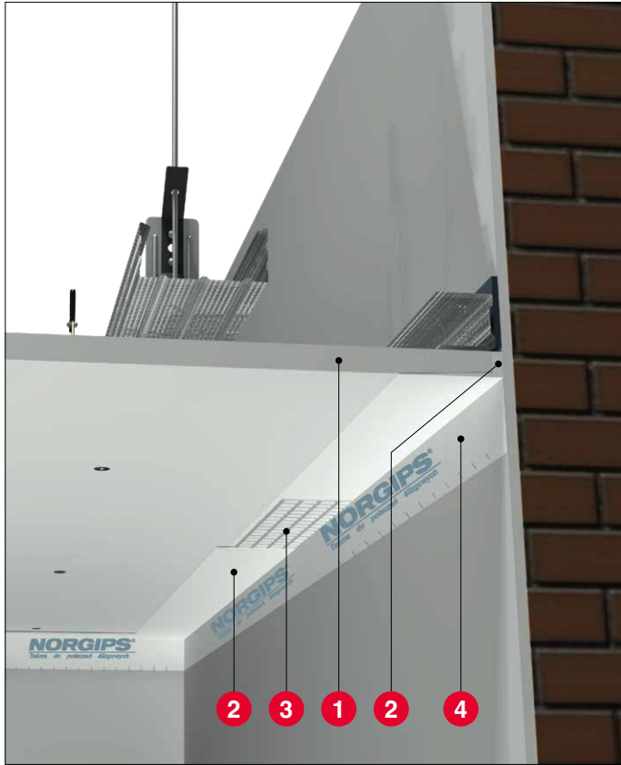
Fig. 5. Sliding joint in a suspended ceiling
