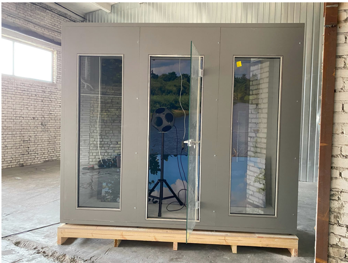
Photo 1. Cabin with sound source inside (front side).
