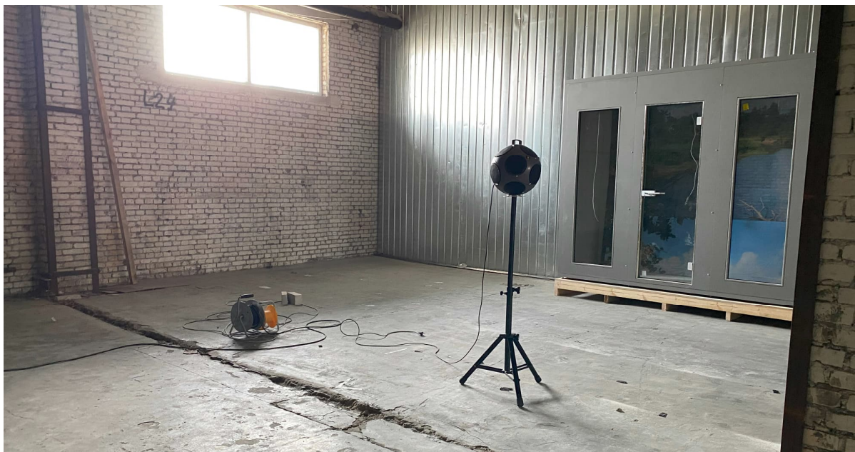
Photo 2. Sound source position without specimen.
